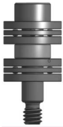
Fig. 111: A sample bearing stack, with a radial bearing sandwiched between 2 thrust bearings on a shoulder screw. A plate (not pictured) rides on the radial bearing while being supported by the thrust bearings.
