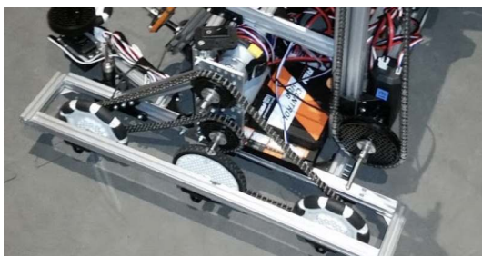
Fig. 29: Properly done chain wrap with the REV system
