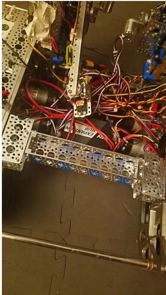
Fig. 1: Bad example of wiring!
