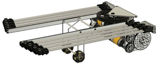
Fig. 48: 11115 Gluten Free, Skystone, round linear bearings and metal shafts with 3D printed mounts
