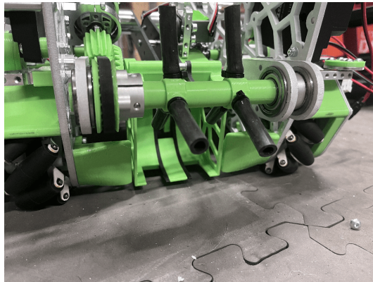
Fig. 96: 16461 Infinite Turtles, Freight Frenzy, Direct transfer intake, where the collection bucket is right behind the intake
