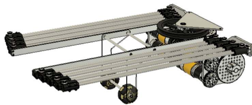
Fig. 48: 11115 Gluten Free, Skystone, round linear bearings and metal shafts with 3D printed mounts
