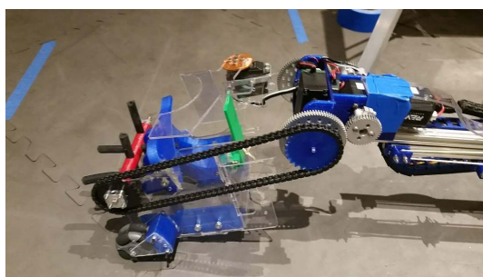
Fig. 28: 9794 Wizards.exe, Rover Ruckus, plastic chain on intake
