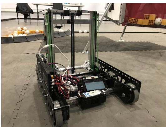
Fig. 50: 7236 Recharged Green, Rover Ruckus, custom box tube linear elevator
