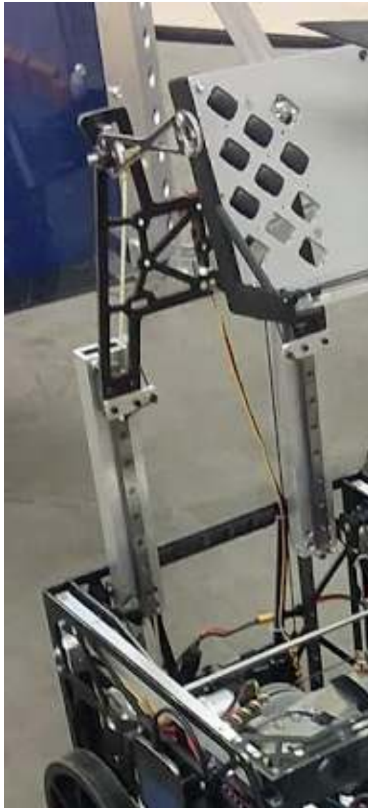
Fig. 44: 8813 The Winter Soldiers, Rover Ruckus, MGN12 slides connected with custom box tubes
