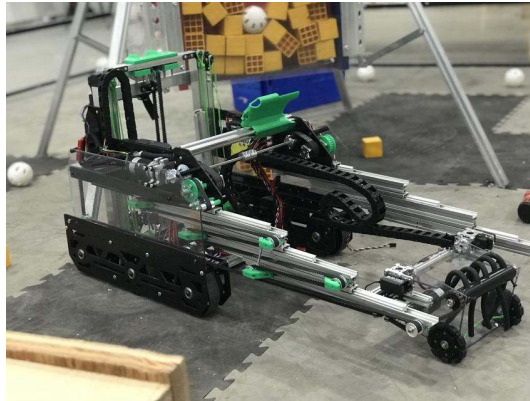
Fig. 66: 7236 Recharged Green, Rover Ruckus: Cable carrier on the left side of their horizontal slides and the right side of vertical slides
