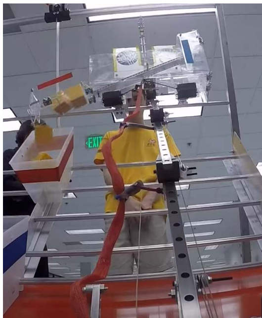
Fig. 45: 8221 Cubix, Res-Q, MGN slides connected with 3D printed parts
