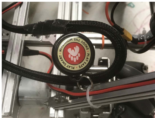
Fig. 68: 248 Fatal Error, Freight Frenzy: Badge retractor cable management on extension mechanism
