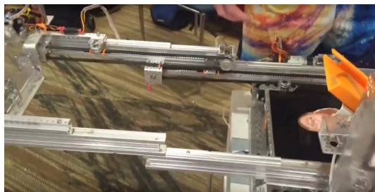
Fig. 63: 5064 Aperture Science Rover Ruckus cascade belt-driven final version
